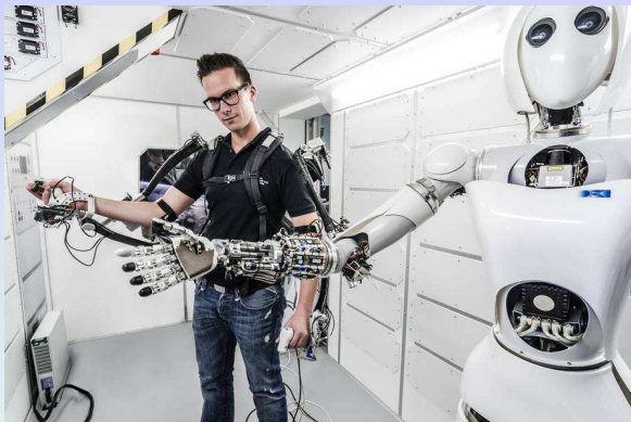
Figura: Exoskeleton-passive: Tele-operation of the human robot Aila, Bremen, Germany.
