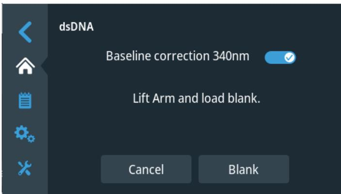
Load blank, close the arm quickly, and select **Blank**.
