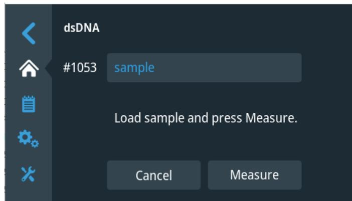
Enter a sample name, load sample, close the arm quickly, and select **Measure** to initiate measurement.
