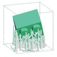
Figura 2: This solid has parts that need support to print correctly. So the printer will build some structures to hold this parts while it is printed.
