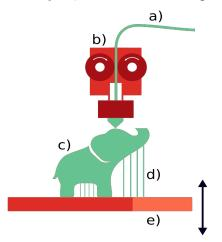
**Figura 1:** A plastic filament (a) is horizontally heated by a controlled nozzle (b), allowing the template (c) to be printed over the horizontal platform (e), that moves on the vertical direction. Some sloping parts of the template need supports (d) to be printed.
